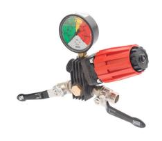
Control unit with working pressure regulating valve, by-pass control lever and glycerine bath pressure gauge with coloured dial. Suitable for AR 503, AR 30 and AR 50 pumps.
