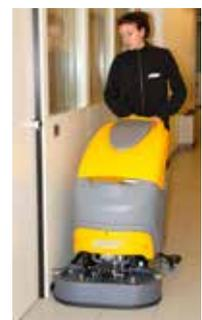
Pivoting wheels under the chassis and their short distance
