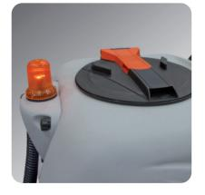
Quick lock recovery tank cap allows for fast and esy cleaning and sanification of the tank; the tilting tank together with a large size drain hose allow the complete emptying of the tank and the removal of any type of solid dirt. The antifoam device protects suction motor, as well as the electronic floating switch that stops suction when the tank is full.
