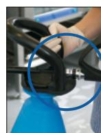
6. The water gun (item no. 93209 or 93219) is connected to the nipple on the injector.
