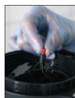
3. Insert the correct nozzle in the injector (see the nozzle directory on the following page).
