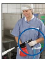
8. Turn on the water tap and start the foam application by pressing the "trigger".
