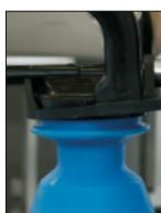
5. Screw the injector tight on the container.
