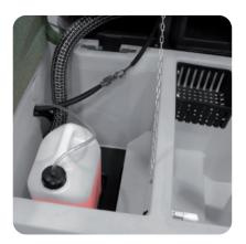
Automatic detergent dosing system (only for model code: 8.525.1301 - 8.525.1302) Fully accessible recovery water tank with visual inspection. Easy access to the recovery tank. Easy access and simple service of the components without use of tools.
