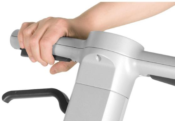
Quick, handy brush coupling and uncoupling: just press the dead man's levers three times then confirm uncoupling on the Vispa EVO display, to remove the brush.
